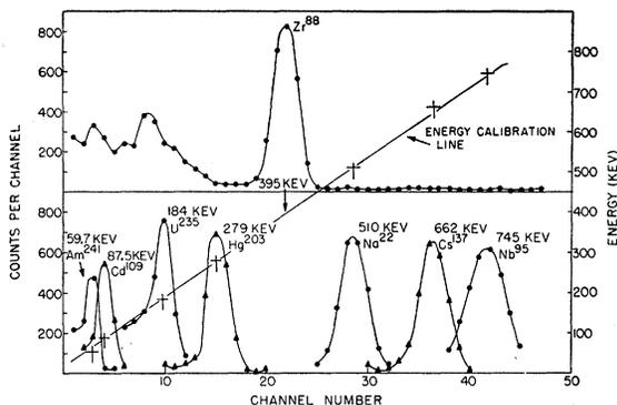
FIG. 1. Gamma spectrum of pure sample of  $Zr^{88}$ .
