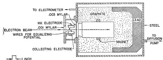
FIG. 1. Schematic drawing of the Faraday-cup beam integrator showing the small ion chamber in front of the mouth of the cup.
