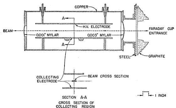
FIG. 3. Configuration of the large ion chamber showing the relative position of the Faraday cup.
