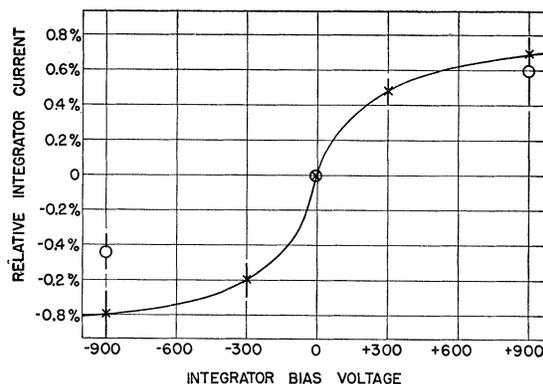
FIG. 2. Integrator response relative to monitor response as a function of the bias voltage applied to the Faraday cup.
