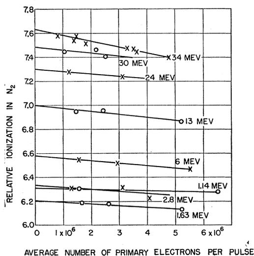
FIG. 4. Ratio of the collected ion charge to collected Faraday-cup charge (in arbitrary units) as a function of the average primary beam intensity.
