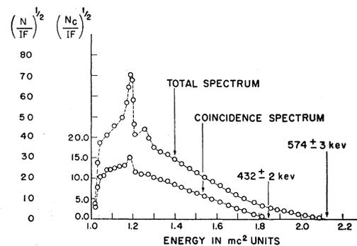
FIG. 2. "Allowed shape" Kurie plots for the total and coincidence beta spectra of  $Ce^{141}$ .
