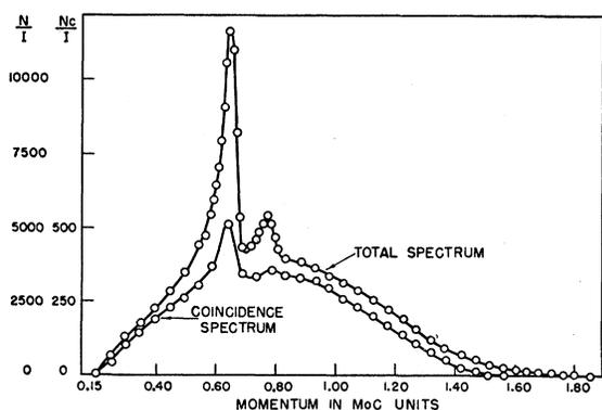
FIG. 1. Total and coincidence beta spectra of  $Ce^{141}$ .  $N$  and  $N_c$  are the number of counts per minute of the total beta spectrum and the coincidence beta spectrum, respectively;  $I$  is the current in the spectrometer coil.
