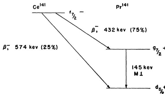
FIG. 4. Decay scheme for Ce<sup>141</sup>.
