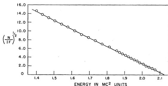
FIG. 3. Kurie plot of the Ce<sup>141</sup> high-energy beta group obtained by subtracting the low-energy beta group from the total beta spectrum.
