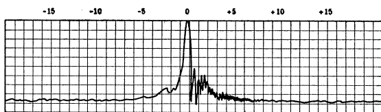
FIG. 2. Proton spectrum at 30 Mc/sec of \text{CH}_3\text{I} enriched with 51 percent \text{C}^{13} with strong 7\frac{1}{2} Mc/sec rf-coupled into the transmitter. The side peaks are almost completely collapsed.
