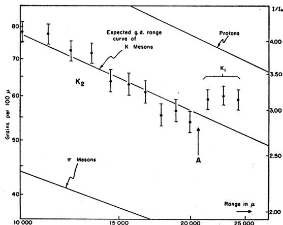
FIG. 2. Grain density vs range measurements (log-log scale) of  $K_2$ . Solid lines: expected curves for protons,  $K$  mesons, and  $\pi$  mesons. (Note: the three points of  $K_1$  are plotted as a function of their distance from the endpoint of  $K_2$ . Therefore, it is not the correct grain density-range plot of  $K_1$ .)
