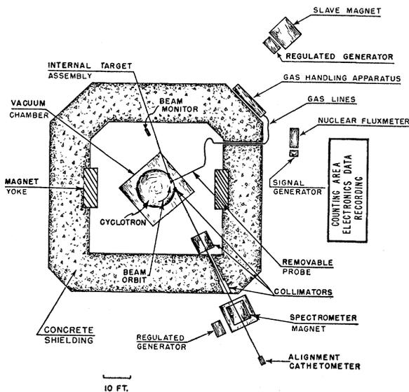
FIG. 4. The general layout of the experimental apparatus.
