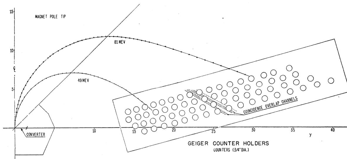
FIG. 7. Top view of counter holder in relation to magnet pole tip. The orbits for 49- and 81-Mev electrons are shown. The overlap channels defined by coincidences between adjacent Geiger tubes are shown for the central energy of the spectrometer. The scale is in inches.
