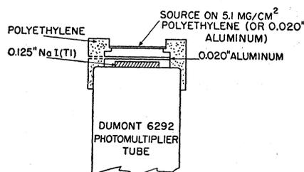
FIG. 2. Schematic diagram of the scintillation counter arrangement.
