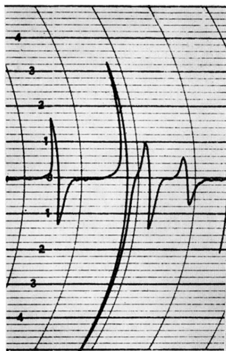
FIG. 1. The above reproduction illustrates typical signals obtained from \text{BaTiO}_3 crystals, in the ferroelectric state corresponding to room temperature, and polarized perpendicular to the direction of the dc magnetic field produced by the V-4007 Electromagnet and V-2200 Power Supply. The resonant frequency of the V-260 Klystron was set at 9.5 kMc/sec.
