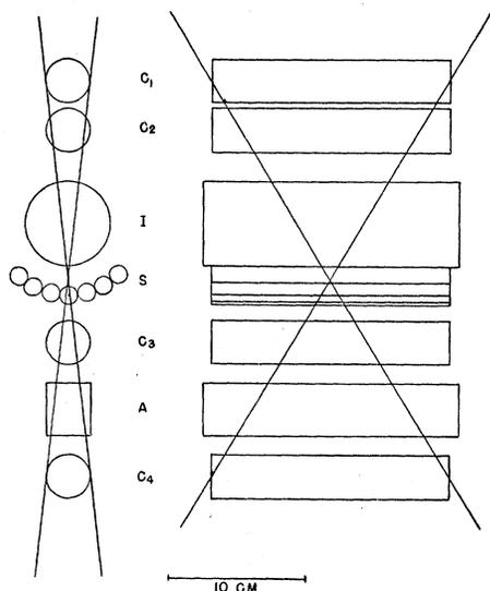
FIG. 1. Diagram of counter telescope.  $C_1$ ,  $C_2$ ,  $C_3$ ,  $C_4$ —G-M counters.  $S$ —shower tray containing seven G-M counters.  $I$ —electron collection ionization chamber.  $A$ —4 cm Pb absorber.
