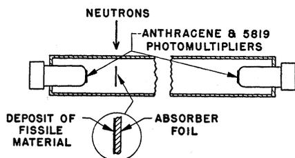
FIG. 1. Schematic diagram of the apparatus used to detect the time of flight of slowed fission fragments. Fragments were slowed by the metal backing of the fissile material. The longest of the drift lengths used was 199 cm and the shortest was 125 cm.
