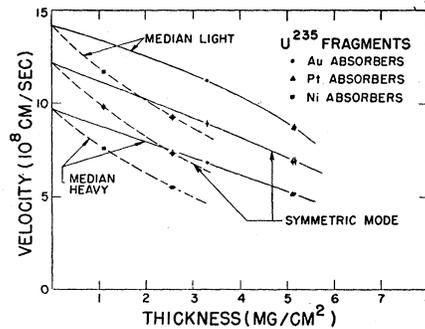
FIG. 3. Range-velocity data of fission fragments in nickel, gold, and platinum. A 3.3-mg/cm<sup>2</sup> gold foil was used in addition to the foils described in the text. Curves are fits of the equation  $dv/dx = -Av^n$  to the data of nickel and gold. When no uncertainties are indicated they are smaller than the datum point.
