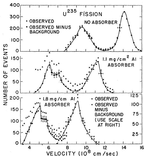
FIG. 5. Velocity distributions of unslowed and aluminum-slowed fragments from  $U^{235}$  fission. Horizontal wings through datum points represent the standard deviations associated with measurement of velocity. Different drift lengths were used in separate measurements of the heavy- and light-fragment groups for 1.8-mg/cm<sup>2</sup> aluminum absorber to improve the velocity resolution of the light fragment group.
