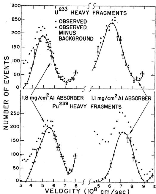
FIG. 6. Velocity distributions of  $U^{233}$  and  $Pu^{239}$  fragments slowed by aluminum. Horizontal wings through datum points represent the standard deviations associated with measurement of velocity.
