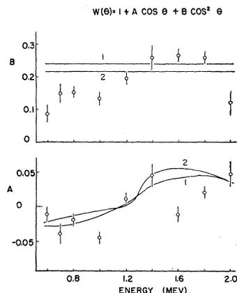
FIG. 3. Energy dependence of the coefficients  $A$  and  $B$  in the expression  $W(\theta) = 1 + A \cos\theta + B \cos^2\theta$  for the yield of 12-Mev gamma rays from the proton bombardment of boron.
