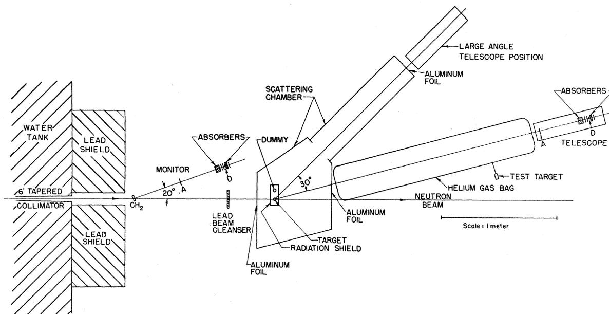
FIG. 1. Schematic diagram of  $n-p$  experiment.
