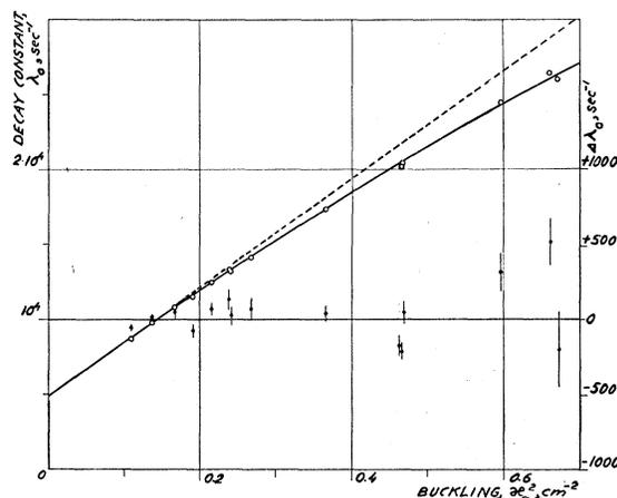
FIG. 2. Measured decay constant  $\lambda_0$  and deviations  $\Delta\lambda_0$  from the parabola  $\lambda_0 = 4907 + 36\,160\kappa_0^2(1 - 0.175\kappa_0^2) \text{ sec}^{-1}$  as functions of the buckling  $\kappa_0^2$ . Vertical lines on the  $\Delta\lambda_0$  points indicate the calculated random errors.
