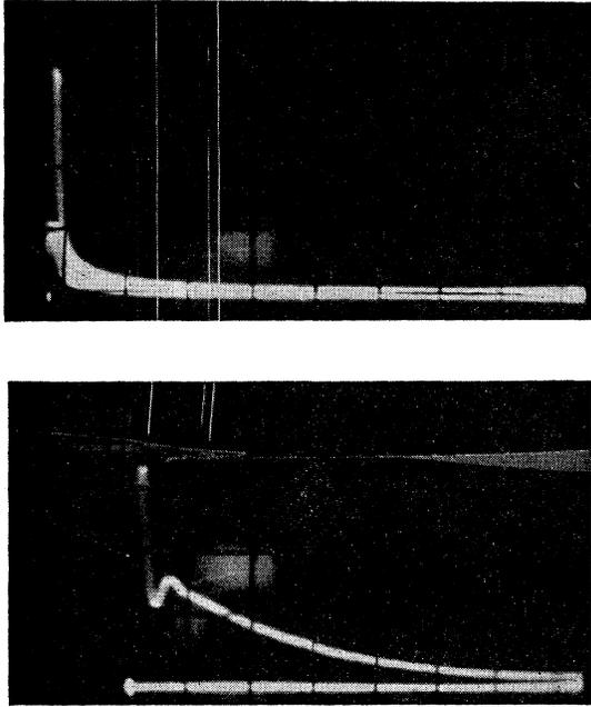
FIG. 1.  $\alpha$ -particle pulses. Experimental conditions as in B. Cathode: nickel well outgassed, 2.9 cm in diameter; argon pressure: 400 mm Hg; corona threshold: 1660 volts; sweep time: 100  $\mu$ sec. The upper pulse, taken 100 volts below the corona threshold, shows the electronic shape of the primary avalanche with no secondary effect. The lower pulse, taken at the corona threshold, shows the peak and the continuous slope due to the diffused photoelectric effect.
