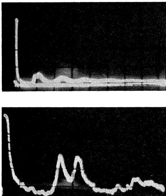
FIG. 3.  $\alpha$ -particle pulses near the corona threshold. Experimental conditions as in B. Argon pressure: 50 mm Hg; corona threshold: 765 volts. The upper pulses, taken with a 2000- $\mu$ sec sweep time, shows the  $\gamma_i$  pulse succession. The first secondary pulse is composed of two distinct peaks due to two different kinds of ions. The lower pulse shows the first part of the upper pulse enlarged. At higher pressure, the separation between the two peaks was not clear.
