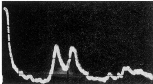
FIG. 3.  $\alpha$ -particle pulses near the corona threshold. Experimental conditions as in B. Argon pressure: 50 mm Hg; corona threshold: 765 volts. The upper pulses, taken with a 2000- $\mu$ sec sweep time, shows the  $\gamma_i$  pulse succession. The first secondary pulse is composed of two distinct peaks due to two different kinds of ions. The lower pulse shows the first part of the upper pulse enlarged. At higher pressure, the separation between the two peaks was not clear.
