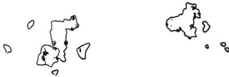
FIG. 11. (a) "Auto-micro-photograph" of two particles of electroluminescent phosphor taken by their own electroluminescence. (Photo by Herndon Associates, Inc., Ipswich, Massachusetts.) (b) Sketch showing approximate outlines of particles illustrated in (a), and approximate locations of "spots."
