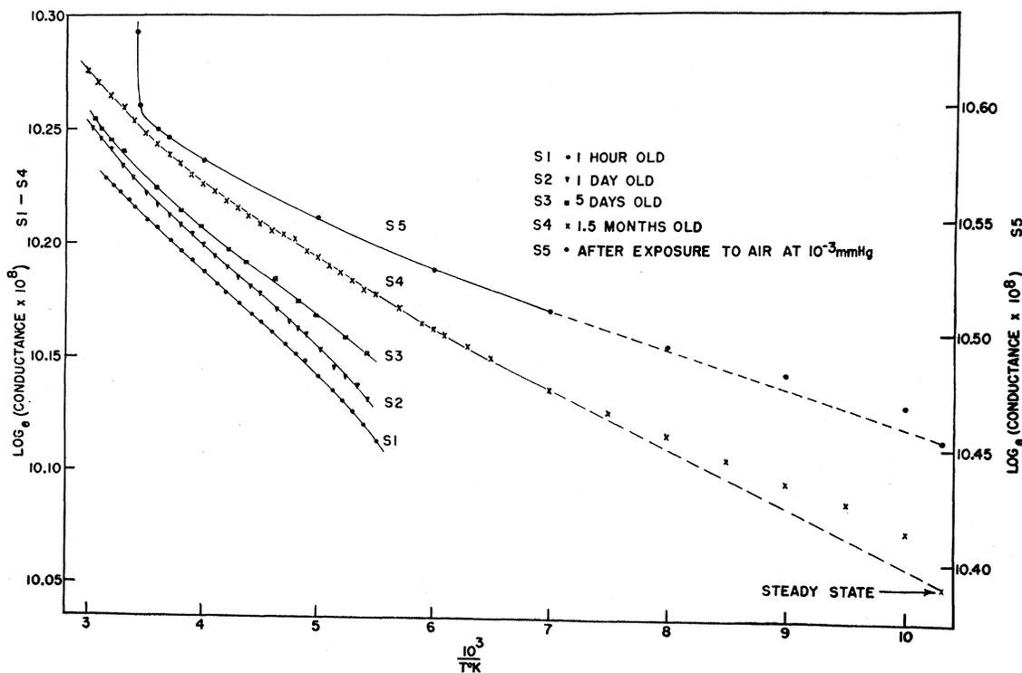
FIG. 1.  $\text{Log}_{10}$  conductance vs  $1/T$  for an alternately evaporated deposit of 210 layers each of iron and lead.
