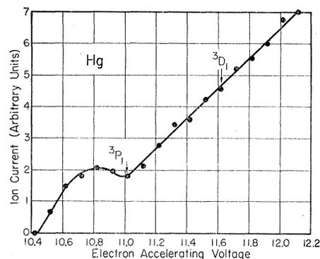
FIG. 5. Relative ionization probability curve for Hg. The states noted are those of Hg I<sup>b</sup>.
