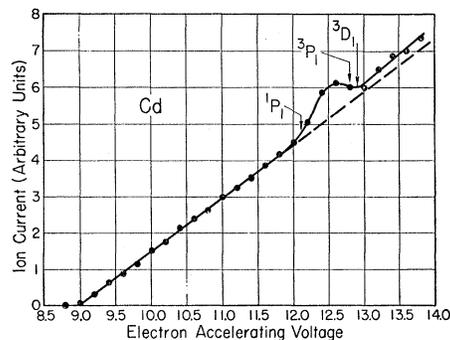
FIG. 3. Relative ionization probability curve for Cd. The states noted are those of Cd I<sup>b</sup>.
