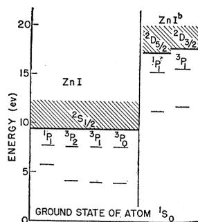
FIG. 2. Simplified energy level diagram for zinc atom. The states arise from the excitation of either a single valence electron (Zn I) or a single inner (*d*) shell electron (Zn I<sup>b</sup>).
