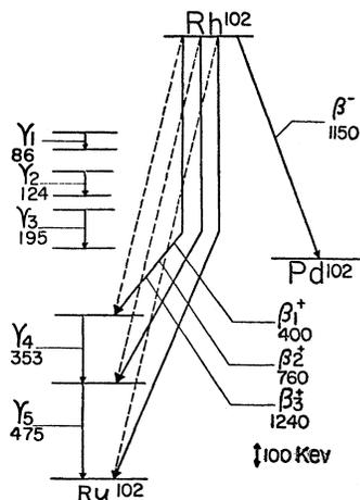
FIG. 4. The incomplete decay scheme of  $Rh^{102}$ .
