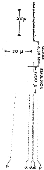
FIG. 4. An oxygen nucleus with energy \sim 60 Bev/nucleon interacts with a nucleus in the glass backing of the emulsion and does not produce a meson shower.
