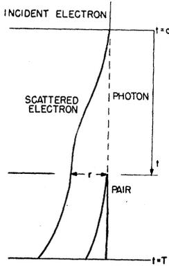
FIG. 2. A schematic diagram to represent the formation of a B.S. pair. The parent electron enters the emulsion at  $t=0$ , at which point the B.S. photon is assumed to originate. The effect of the angles of emission in the radiative collision has been neglected. At  $t$  the photon forms a pair and the parent electron has been scattered away a distance  $r$ , leaving the emulsion at  $t=T$ .
