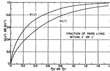
FIG. 3. The fraction of B.S. pairs formed within a projected distance  $x'$  or radial distance  $r'$  from the track of the parent electron as a function of the dimensionless variables  $\eta_{x'}$ ,  $\eta_{r'}$ , respectively.
