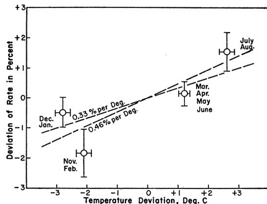
FIG. 1. Percent deviations of average counting rates from the over-all mean, as a function of the deviations of effective atmospheric temperature. The line drawn with a slope of 0.33 percent per degree is the least squares solution for these data; the line drawn at 0.46 percent per degree represents the result of combining the present data with a previous measurement.
