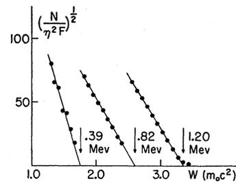
FIG. 2. Fermi plot for Sc<sup>43</sup>.
