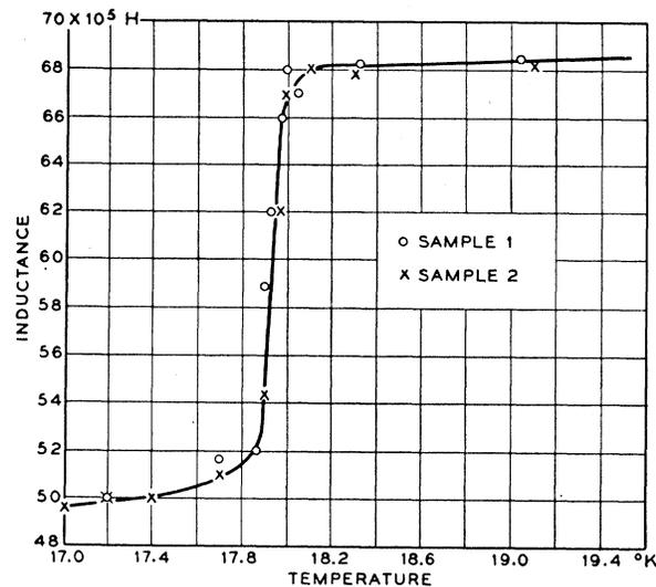
FIG. 1. Variation of susceptibility with temperature of Nb<sub>3</sub>Sn.
