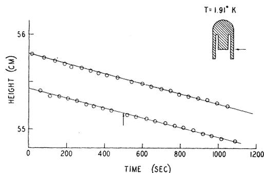
FIG. 2. The height of the meniscus and bath (lower curve) as a function of time for an annular capillary 100 microns wide. The arrow indicates the point at which the evaporating bath just reaches the bottom of the annular space. Temperature  $1.91^{\circ}\text{K}$ .
