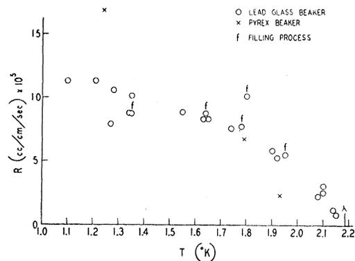
FIG. 4. The film transfer rate ( $R$ ) as a function of temperature deduced from the capillary beaker experiments.
