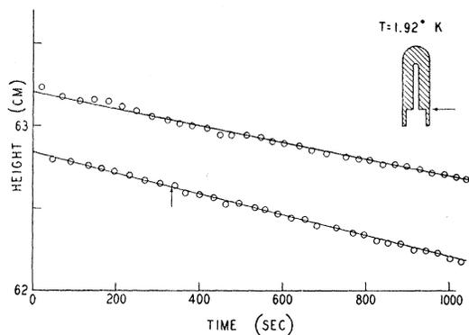
FIG. 1. The height of the meniscus and bath (lower curve) as a function of time for a circular capillary 226 microns in diameter. The arrow indicates the point at which the evaporating bath just reaches the bottom of the capillary. Temperature  $1.92^{\circ}\text{K}$ .
