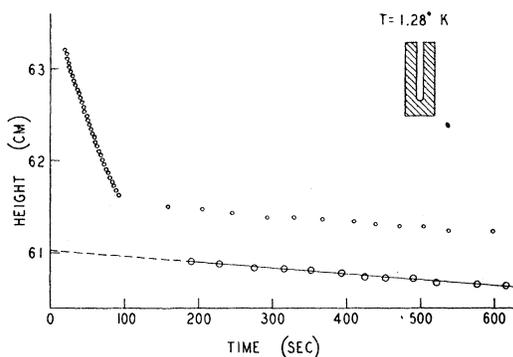
FIG. 3. An "emptying" process for a 185-micron circular capillary beaker. The bath level (lower curve, large circles) was, at all times, in contact with the outside of the beaker. Temperature  $1.28^{\circ}\text{K}$ .
