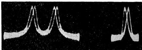
FIG. 1. Oscilloscope pictures of resonance absorption in lithium vs magnetic field. *Left*: Electron spin resonance. Zero field at the center of the sweep. The four peaks arise from a small phase shift between the horizontal and vertical axes. Sweep amplitude about 40 gauss. *Right*:  $\text{Li}^7$  nuclear resonance at about 10 000 gauss. Sweep amplitude approximately 3 gauss.
