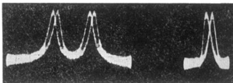
FIG. 1. Oscilloscope pictures of resonance absorption in lithium vs magnetic field. Left : Electron spin resonance. Zero field at the center of the sweep. The four peaks arise from a small phase shift between the horizontal and vertical axes. Sweep amplitude about 40 gauss. Right : Li^7 nuclear resonance at about 10 000 gauss. Sweep amplitude approximately 3 gauss.
