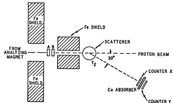
FIG. 2. Geometry for the second scattering.
