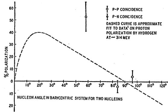
Fig. 9. Polarization of a nucleon scattered by a quasi-free nucleon-nucleon collision vs angle in the barycentric system of two nucleons. The  $p-n$  polarization value is plotted at the angle of the scattered neutron.
