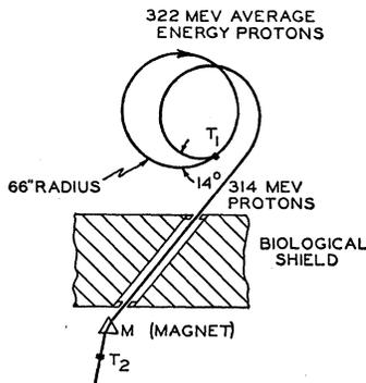
FIG. 1. Plan view of 450-Mev synchrocyclotron area, showing the experimental arrangement used to produce a 314-Mev proton beam, about 60 percent polarized in the vertical direction.
