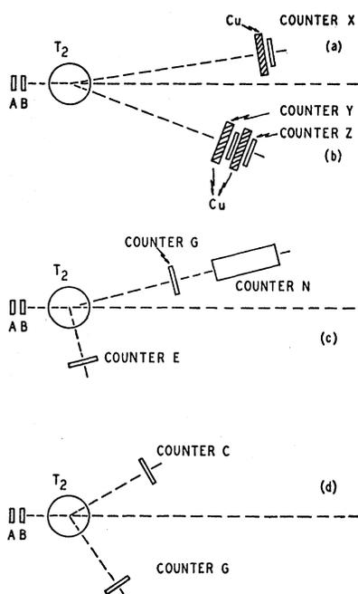
FIG. 3. Various arrangements of counter telescopes to detect scattered particles.
