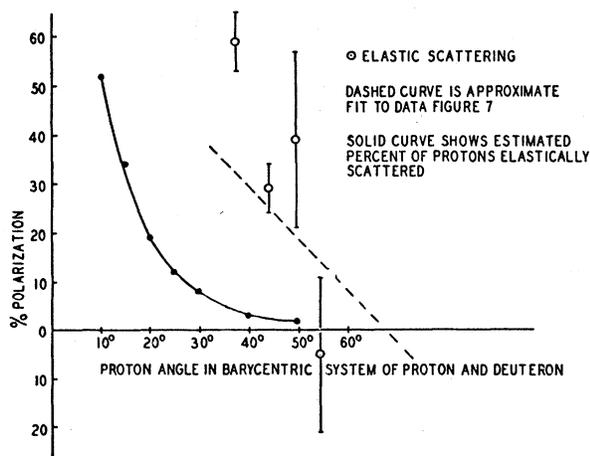
Fig. 8. P, Polarization vs angle in the  $p-D$  center-of-mass system for protons scattered by deuterium. For these measurements the detecting counters had copper absorbers in front which excluded nearly all particles except protons elastically scattered from deuterium. However, at angles less than  $30^\circ$  the discrimination is incomplete.
