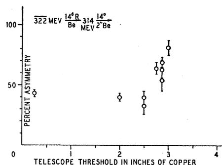
FIG. 5. Asymmetry vs energy threshold of the detecting counters. First scattering, 322-Mev *p* on Be, at  $14^\circ$  to the right. Second scattering, 314-Mev *p* on Be, at  $14^\circ$ .
