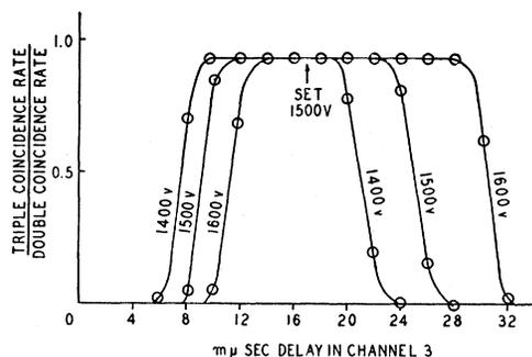
FIG. 4. Coincidence delay curves. Photomultiplier plateaus vs relative delay.
