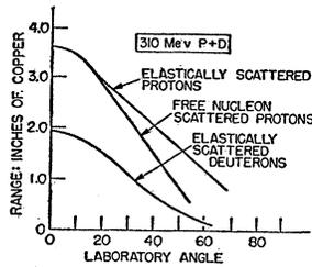
Fig. 7. Range in copper of the scattered particles. Upper curve: protons from elastic  $p-d$  collisions. Center curve: protons scattered by a free nucleon. Lower curve: deuterons from  $p-d$  scattering.
