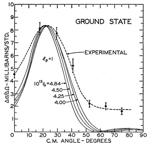
FIG. 6. Experimental and (smeared) theoretical angular distributions for the ground-state  $B^{10}(n,d)Be^9$  reaction.
