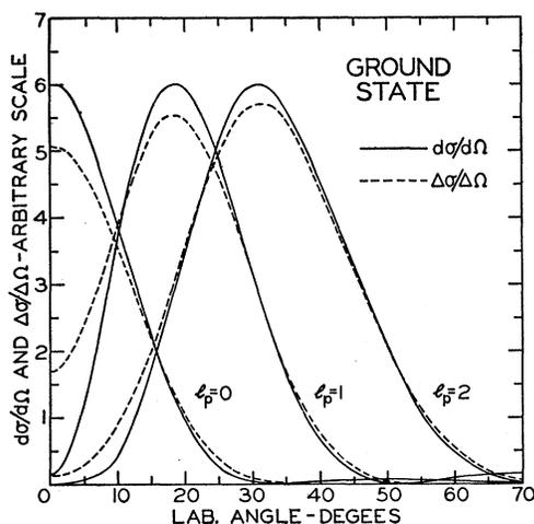
FIG. 3. Theoretical angular distributions for the ground-state  $B^{10}(n,d)Be^9$  reaction (solid curves) and the corresponding distributions modified by the effect of finite angular resolution (dashed curves).
