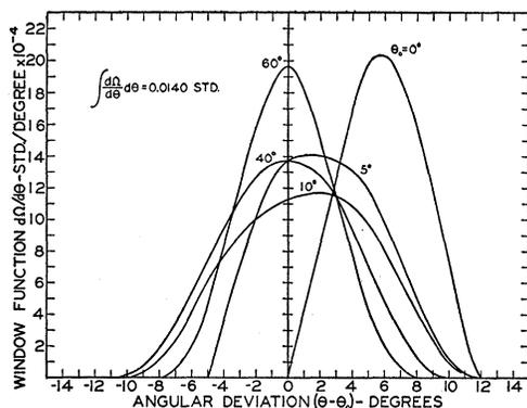
FIG. 2. Window function for counter-telescope spectrometer, showing the effect of finite angular aperture for various angular settings  $\theta_0$  of the spectrometer axis.
