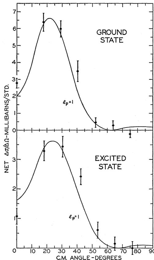
FIG. 8. Comparison with theory of experimental angular distributions after subtraction of isotropic components.
