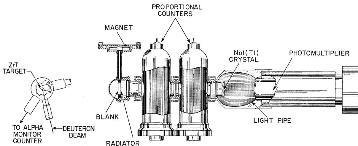
Fig. 1. Apparatus for measuring the  $B^{10}(n,d)Be^9$  cross sections, showing  $T(d,n)He^4$  neutron source and coincidence-telescope spectrometer.
