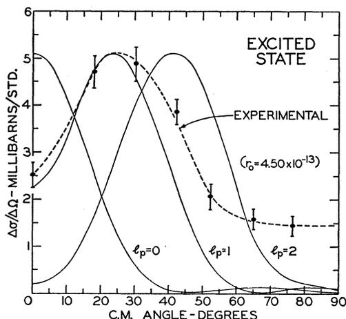
FIG. 7. Comparison of the experimental angular distribution for the excited-state deuteron group with the (smeared) theoretical curves corresponding to various values of the orbital angular momentum of the picked-up proton.
