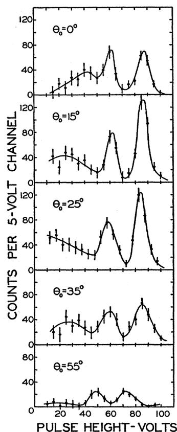
FIG. 4. Scintillator pulse-height distributions for the charged reaction products from the interaction of 14-Mev neutrons with  $B^{10}$ , for various spectrometer (laboratory) angles.
