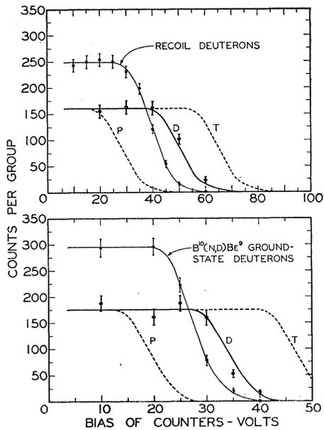
FIG. 5.  $dE/dx$ -bias curves used to identify the two principal charged-particle groups as deuterons. The upper curve in each graph corresponds to deuterons of known energy. The lower curves are calculated for the particles in question, assuming them to be either protons, deuterons, or tritons.
