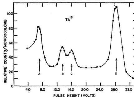
FIG. 1. The pulse-height distribution obtained for the radiation from a 5-mil tantalum target bombarded with 3-MeV protons using a 1-mm gold absorber. Peak A corresponds to the tantalum K x-ray. Peaks B, C, and D correspond to gamma rays of 139, 167, and 309 keV.
