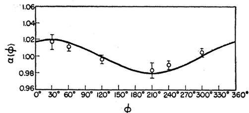
FIG. 7. Asymmetry in intensity as a function of direction, after scattering by a gold polarizer and a silver analyzer.
