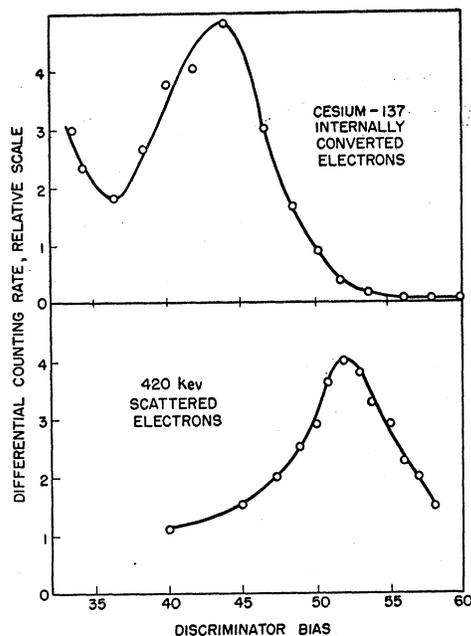
FIG. 4. Discriminator curves after differentiation. The abscissa scales of the two curves are not directly comparable, because the amplifier gains were not the same.
