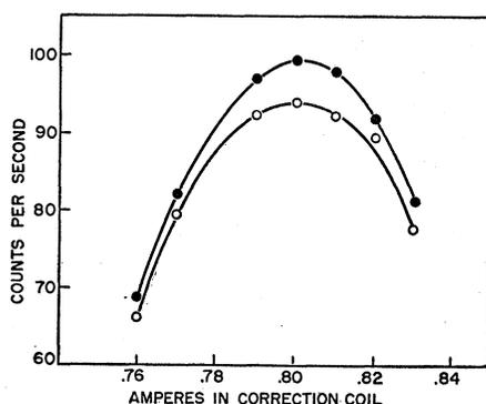
FIG. 3. Typical plot used for centering the beam on the analyzer foil. Circles and dots refer to the two counters. Cyclotron rotation, 1814 degrees.
