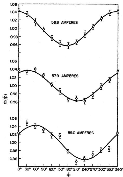
FIG. 6. Asymmetry in intensity as a function of direction, after scattering by a gold polarizer and a gold analyzer.
