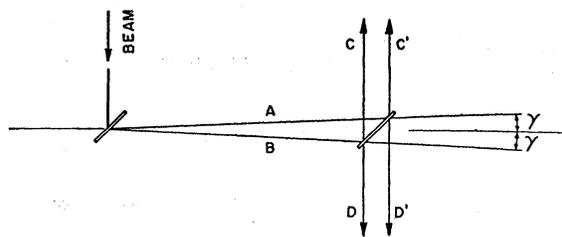
FIG. 5. The introduction of a nonspin asymmetry in the double-scattering experiment by a finite aperture.
