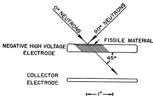
FIG. 1. Schematic representation of the fission chamber.
