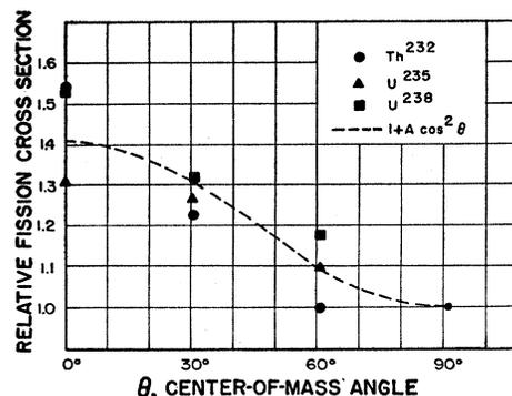
FIG. 2. Angular distribution of fragments from the 14-Mev fission of  $\text{Th}^{232}$ ,  $\text{U}^{235}$ , and  $\text{U}^{238}$ .
