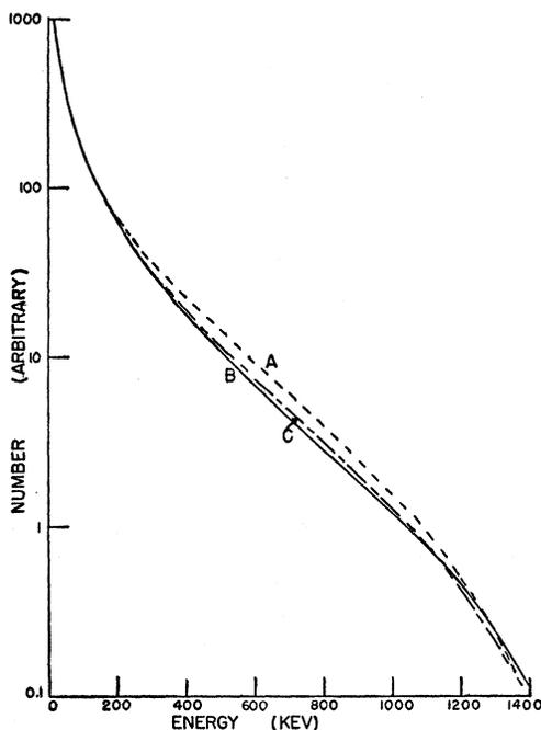
FIG. 1. Calculated energy distributions of internal bremsstrahlung resulting from three beta-interactions (A) allowed; (B) first-forbidden; scalar; (C) first-forbidden; tensor;  $\Delta J=2$ , yes. The ordinates are normalized to 100 at 150 keV. The calculations are made from equations given in reference 4.
