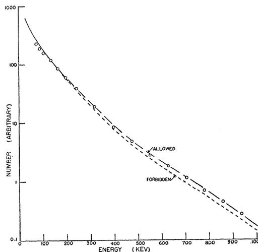
FIG. 2. Energy distribution of internal bremsstrahlung from  $P^{32}$ . The dashed curves are the calculated spectra for allowed and first-forbidden (tensor) beta interactions shown in Fig. 1 corrected for detector response. The circles are the experimental points. Standard error from counting statistics is less than the size of the points. Calculated curves and experimental data have been normalized to 100 at 150 keV.
