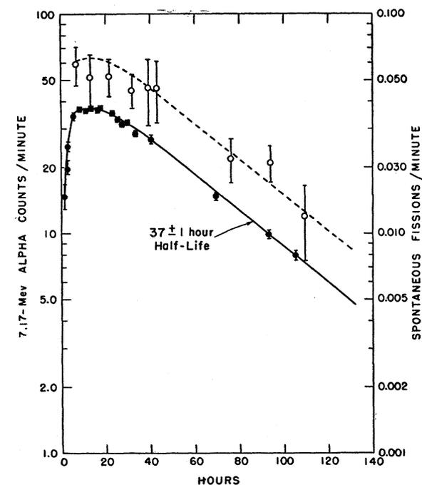
FIG. 3. Growth and decay of element-100 isotope in an initially separated element-99 fraction. The solid circles represent the 7.17-Mev alpha activity on drop 71 as a function of time. The open circles represent the spontaneous fission activity on drop 68 as a function of time. The dashed line is a parallel displacement of the solid line.
