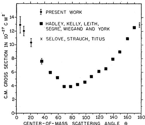
FIG. 2. Differential neutron-proton cross section in the center-of-mass system in  $10^{-27}$  cm<sup>2</sup>/steradian.
