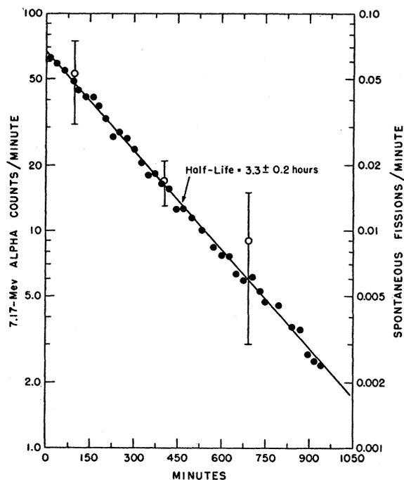
FIG. 2. Decay of the element-100 fraction. The solid points represent the 7.17-Mev alpha counts/minute of drop 60 as a function of the time in minutes. The open circles represent the spontaneous fission activity of drop 61 as a function of time.
