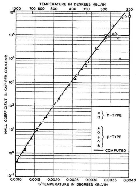
FIG. 6. Hall coefficient vs reciprocal temperature.
