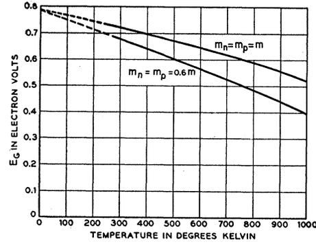
FIG. 7. Intrinsic ionization energy vs temperature.
