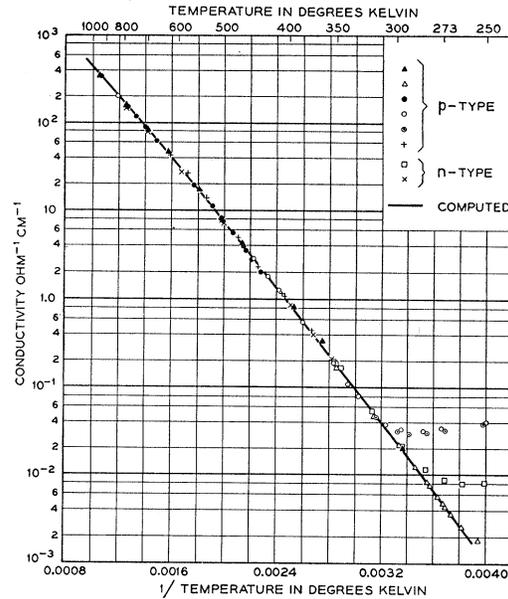
FIG. 2. Conductivity vs reciprocal temperature.
