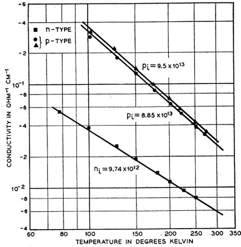
FIG. 3. Conductivity vs temperature in the range where carrier concentration is constant.
