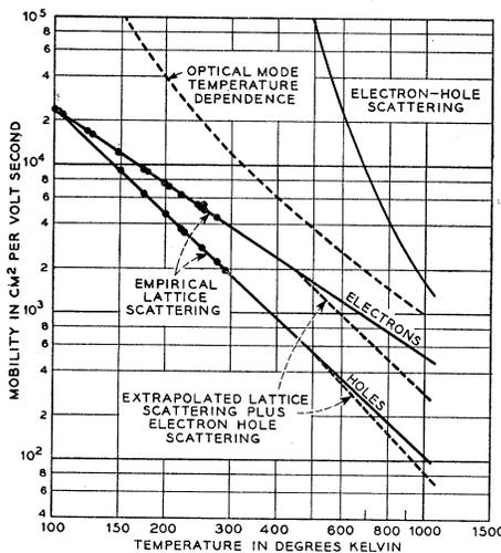
FIG. 1. Conductivity mobility vs temperature.
