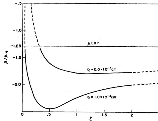
FIG. 4. Magnetic moment of  $K^{40}$  as a function of spin-orbit parameter  $\zeta$  for Gaussian potential and various ranges. For scale and notation see Fig. 2.
