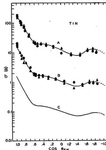
FIG. 2. Angular distribution of 3.7-Mev neutrons scattered from tin: (A) apparent differential cross section using 1-in. axial thickness ring scatterers; (B) apparent differential cross section using  $\frac{3}{8}$ -in. axial thickness ring scatterers; (C) true differential cross section for elastic scattering obtained by a point-by-point linear extrapolation of curves (A) and (B) to zero-thickness scatterer. Remarks concerning ordinates are the same as in Fig. 1.
