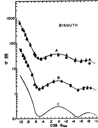
FIG. 3. Angular distribution of 3.7-Mev neutrons scattered from bismuth: (A) apparent differential cross section using 1-in. axial thickness ring scatterers; (B) apparent differential cross section using  $\frac{3}{8}$ -in. axial thickness ring scatterers; (C) true differential cross section for elastic scattering obtained by a point-to-point linear extrapolation of curves (A) and (B) to zero-thickness scatterer. Remarks concerning the ordinates are the same as in Fig. 1.
