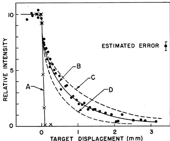
Fig. 1. Intensity of 114-keV gamma radiation as a function of the distance travelled by the fluorine recoils before radiating. Curve A is obtained by stopping all recoils at the target in an additional nickel foil. Curves B, C, and D are computed for mean lifetimes of  $10^{-9}$  sec,  $1.5 \times 10^{-9}$  sec, and  $0.66 \times 10^{-9}$  sec, respectively.
