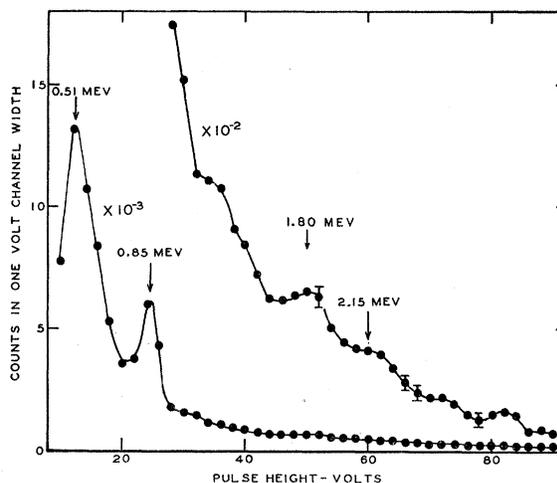
FIG. 4. Gamma-ray spectrum excited by the scattering of 3.9-Mev neutrons in iron.
