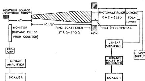
Fig. 1. Geometry and instrumentation for the detection of gamma rays excited by inelastic scattering of neutrons.
