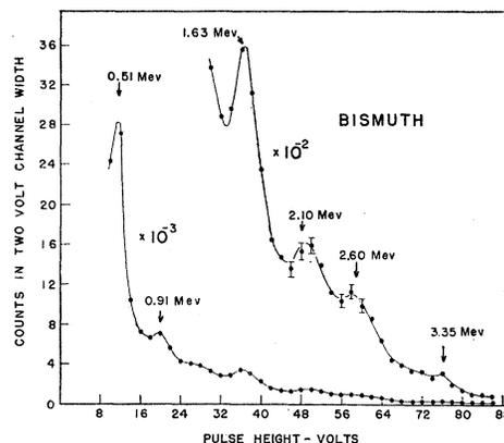
FIG. 3. Pulse-height distribution generated in the crystal of NaI-Tl by the gamma rays resulting from the inelastic scattering of 3.9-Mev neutrons in bismuth.
