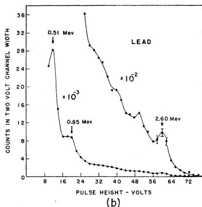
FIG. 2. The energy distribution of pulse heights in the crystal of NaI-Tl with carbon and lead scatterers are shown in Fig. 2(a). Taking the carbon curve as background, the supposed actual contribution of the lead scatterer is shown in Fig. 2(b).
