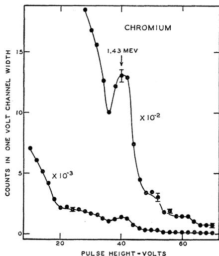
FIG. 6. Gamma-ray spectrum excited by the inelastic scattering of 3.9-Mev neutrons by chromium.
