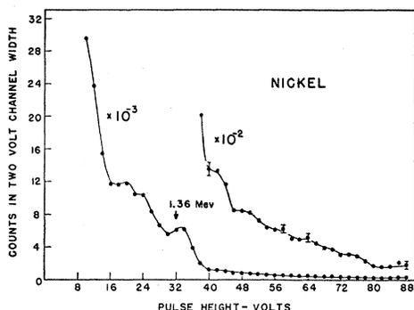
FIG. 5. Gamma-ray spectrum excited by 3.9-Mev neutrons on nickel.
