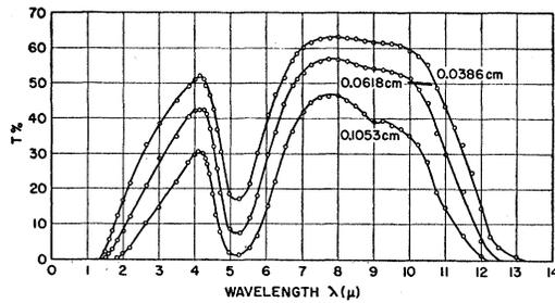
Fig. 1. Transmission spectrum of NiO from  $1\mu$  to  $14\mu$  for sample thickness  $0.1053\text{ cm}$ ,  $0.0618\text{ cm}$ , and  $0.0386\text{ cm}$ .
