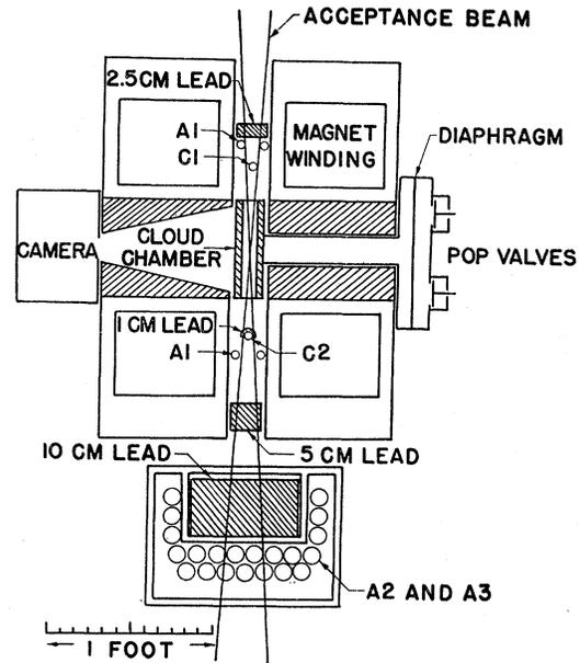
FIG. 1. Sketch of experimental apparatus.
