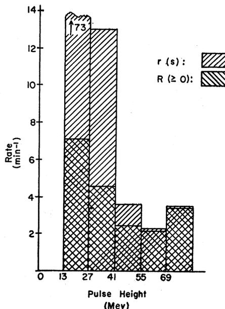
FIG. 8. Comparison of the rate of detected disintegrations, calculated from  $r(s,n)$  and  $r(s,2n)$ , with the observed scintillation rate.
