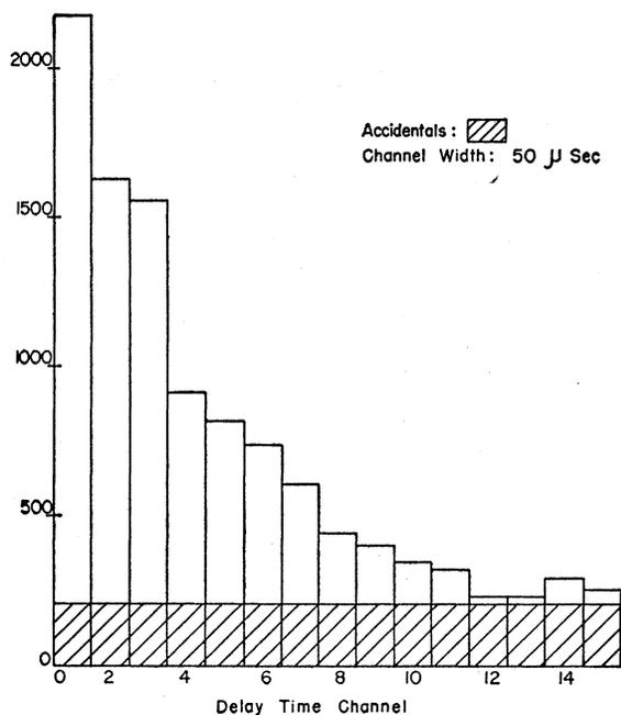
FIG. 4. Distribution of delay times for  $(s,n)$  coincidences. The channel width is 50 microseconds.
