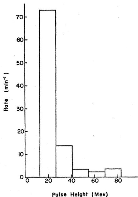
FIG. 5. Scintillation pulse-height distribution.
