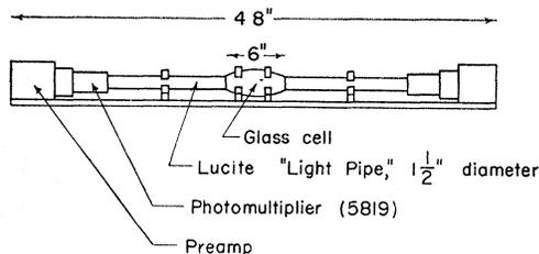
Fig. 2. Scintillator and photomultiplier assembly.
