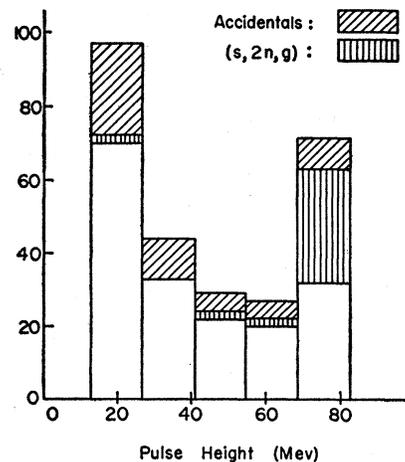
FIG. 7. Pulse-height distribution of  $(s,2n)$  and  $(s,2n,g)$  coincidences.
