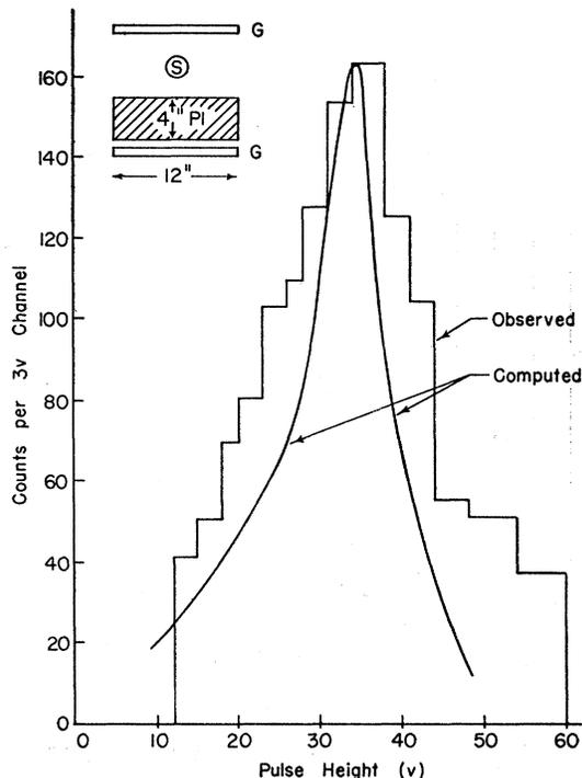
Fig. 3. Pulse-height distribution of minimum-ionizing particles.
