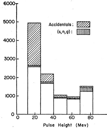
FIG. 6. Pulse-height distribution of  $(s,n)$  and  $(s,n,g)$  coincidences.
