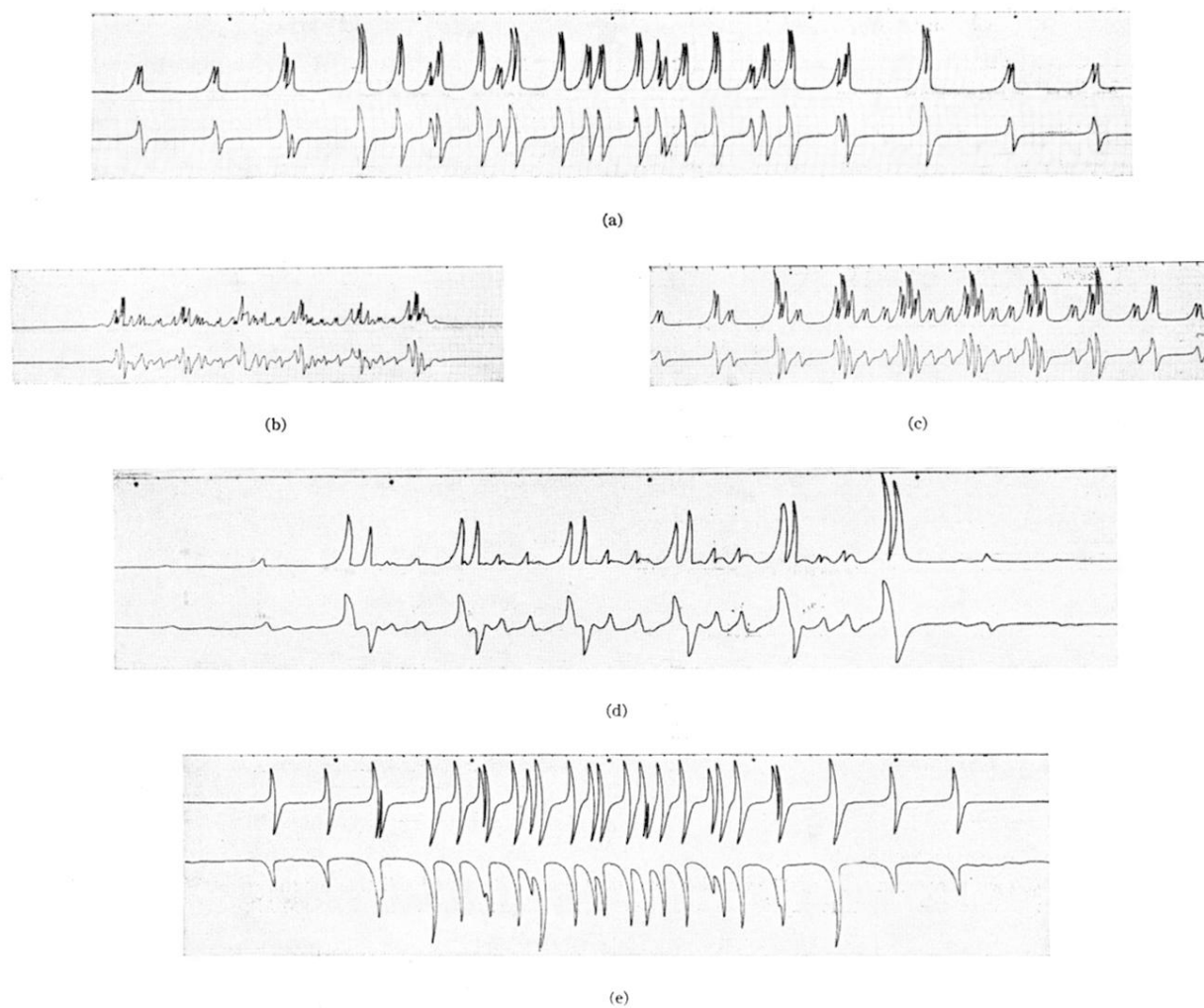
FIG. 2. Experimental records for \text{CaCO}_3:\text{Mn} 0.06 wt. percent. (a) \theta=0^\circ ; (b) \theta=57^\circ ; (c) \theta=90^\circ ; (d) powdered; (e) \theta=0^\circ . R_f=9300 Mc/sec. The slope of the absorption curve is recorded except in the lower \theta=0^\circ case where the relationship between the slope and direct absorption is shown. The magnetic field markers appear at the top of the records.
