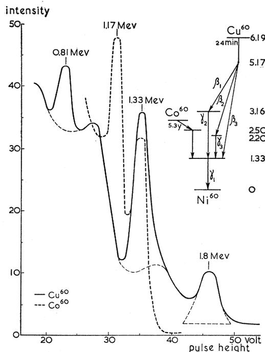
FIG. 1.  $\gamma$ -ray spectra of  $\text{Cu}^{60}$  and  $\text{Co}^{60}$ , taken with a 1-in. NaI crystal mounted on a Dumond K-1186 photomultiplier tube. The decay characteristics of the proposed decay scheme are given in Table I.
