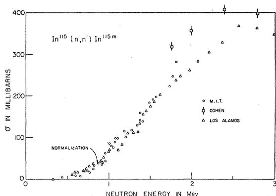
FIG. 2. Neutron excitation of  $\text{In}^{115m}$ . The uncertainty in the energy assignments for our data is about 40 kev. The early data of Cohen (reference 1) and the recent data from Los Alamos (reference 7) have been used to obtain the cross-section scale. Our data have been normalized with those from Los Alamos at 0.88 Mev. The agreement between the data is fairly good but not quite as good as in the case of  $\text{Au}^{197m}$ .
