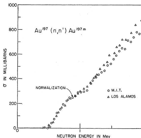
FIG. 1. Neutron excitation of  $\text{Au}^{197m}$ . The Los Alamos results have been plotted after normalization of the two sets of data at 0.88 Mev. In general the agreement is quite good. Our data indicate levels at 1.14 and 1.44 and possibly at 1.7 Mev which are not evident in the Los Alamos data.
