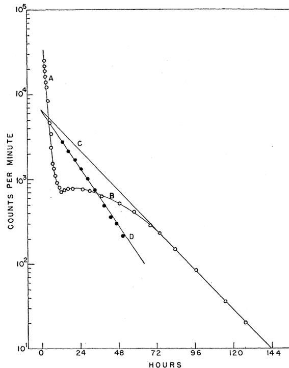
FIG. 1. Open circles—observed activity. Solid circles—subtraction of observed curve from extrapolated asymptote. Curve A, decay of 1.1-hour  $\text{Kr}^{77}$ . Curve B, growth and decay of  $\text{Br}^{76}$ . Curve C, extrapolated asymptote to curve B. Curve D, difference curve obtained by subtracting curve B from curve C. Curve D shows a half-life of  $(9.7 \pm 0.5)$  hours for  $\text{Kr}^{76}$ .
