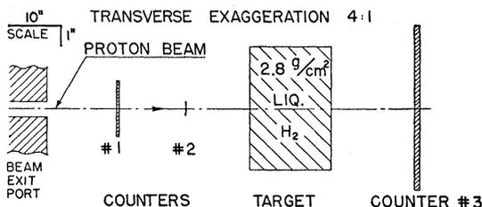
FIG. 1. Schematic diagram of the experimental geometry.
