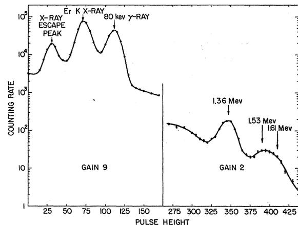
FIG. 1. Pulse-height distribution of  $\gamma$ -ray spectrum observed with  $\text{NaI}(\text{Tl})$  scintillation counter. Note the change in pulse-height scale and amplifier gain for high-energy region.
