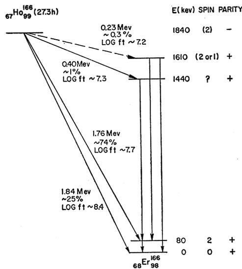
FIG. 3. Disintegration scheme for  $\text{Ho}^{166} \xrightarrow{\beta^-} \text{Er}^{166}$ .
