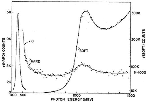
FIG. 1. The excitation function for the various  $\gamma$  rays from the reaction  $\text{Li}^7 + p$ . The soft  $\gamma$  rays are from  $\text{Li}^7(p, p'\gamma)\text{Li}^7$ . The hard  $\gamma$  rays are from  $\text{Li}^7(p, \gamma)$ .
