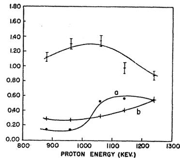
FIG. 9. Angular distribution coefficients of the hard  $\gamma$  rays from  $\text{Li}^7(p, \gamma)$ . The angular distributions are of the form  $W(\theta) = W(\pi/2)[1 + a \cos\theta + b \cos^2\theta]$ . The coefficient  $W(\pi/2)$  is divided by 100.
