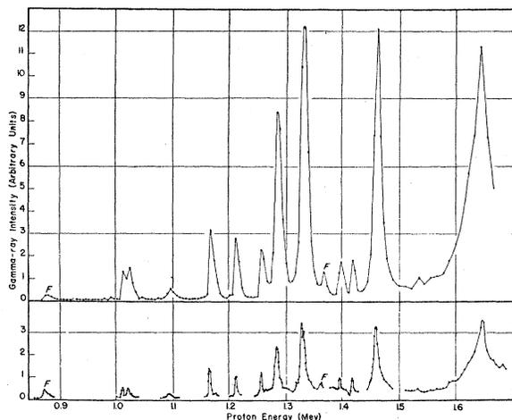
Fig. 2. The γ-ray yields observed when thin sodium targets were bombarded with protons. The upper yield curve was observed using targets prepared by heating tungsten sheet in an oxygen atmosphere. Sodium was found in the oxide layer thus formed. The lower yield curve was observed with use of targets prepared by vacuum evaporation of sodium onto tungsten backing material. The peaks labeled *F* are primarily the result of slight fluorine contamination of the targets.
