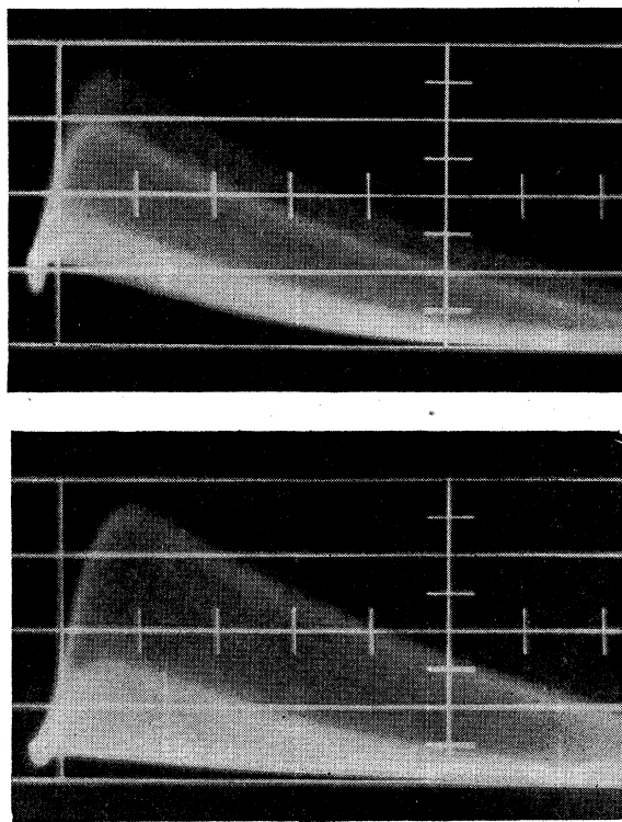
FIG. 3. Thick target pulse-height distributions resulting at proton bombarding energy of 1.07 Mev. The photograph on top was obtained with an enriched B^{10} target. The photograph below was obtained under identical conditions with an elemental boron target.
